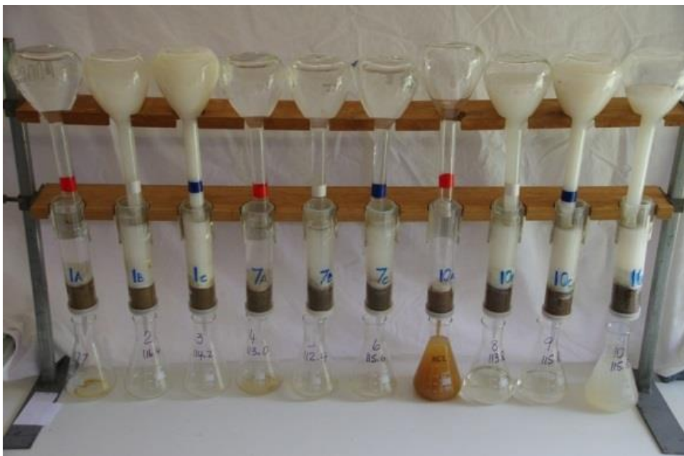
Figure 1 Setup of leachate column trial
